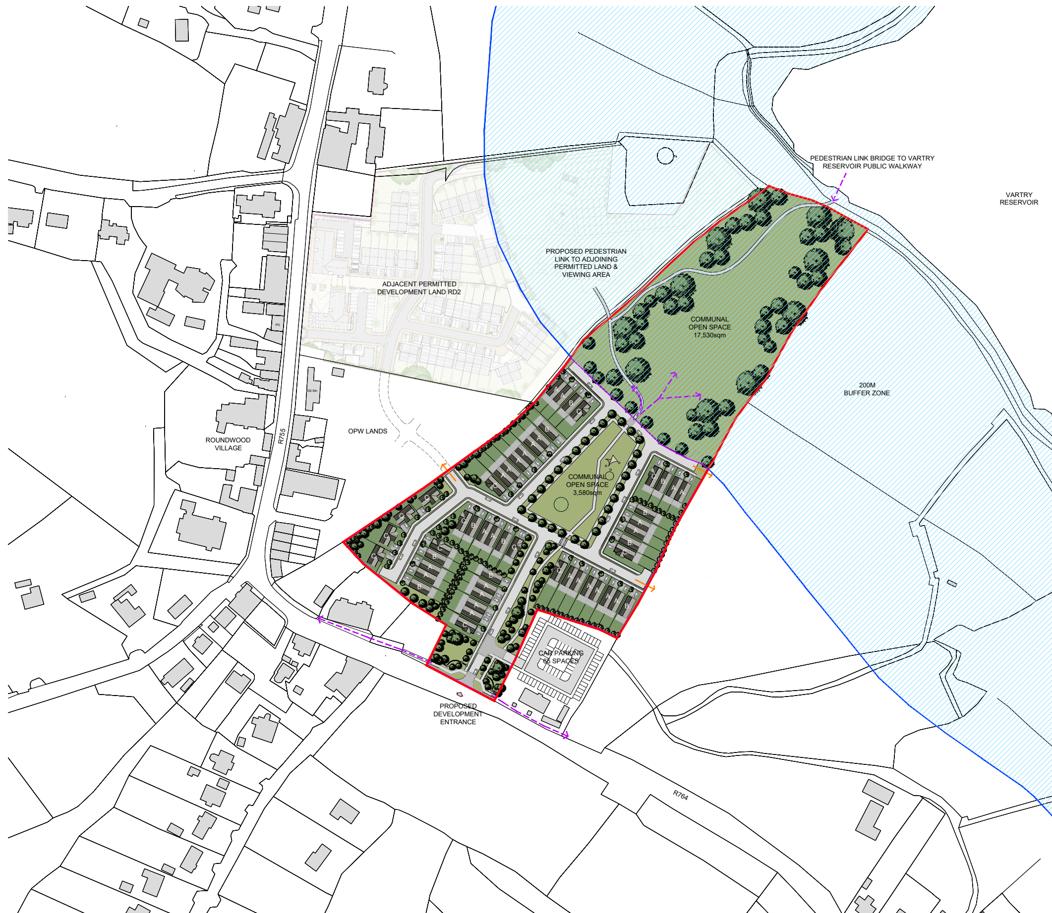
PROPOSED SITE PLAN WITH 200M BUFFER ZONE FROM RESERVOIR SHOWN 1:2500 @ A3
