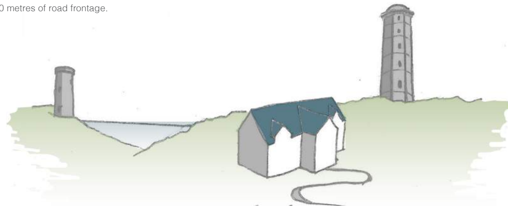
Avoid building in prominent open areas, or areas of protected views or landscapes.
